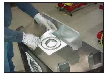
Figure 7.4 Remove the vent cap.
